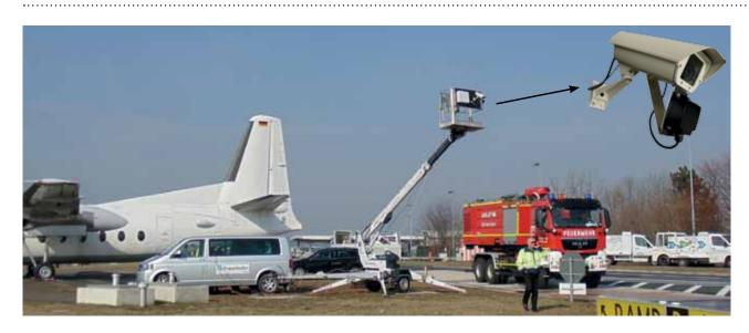
IMST GmbH and the Fraunhofer Institute for Communication, Information Processing and Ergonomics (FKIE) made a radar/video test campaign at the airport Cologne/Bonn. The system controls airport supply vehicle traffic that must cross the aircraft taxiway. If the sensors detect any objects (e.g. suitcases or other goods in transit), persons or vehicles, the intersection will remain closed to aircrafts until the areas has been cleared.
